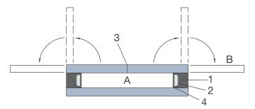
Prepare a small sample of IG unit +/- 200 mm x 200 mm, spacer and butyl only on 2 sides.
