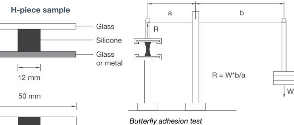
The butterfly adhesion test is an alternate procedure to evaluate adhesion of the sealant to glass. This test can be performed as an alternative or in addition to the H-piece test. This test may be performed on a test mock up sample or directly on an actual IG production unit — always use representative samples of all substrates.
