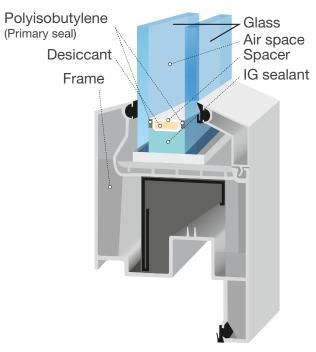
glass sealants which are recommended for nonstructural and structural applications can be used effectively in these designs.
