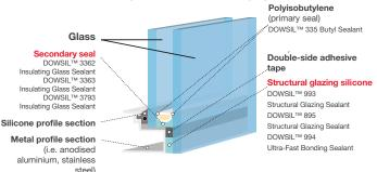
Since these designs are proprietary to the system designer, Dow reviews and approves these designs on a system by system basis. Although the designs may appear similar, variations will determine whether Dow considers the design a "structural glazing" or an "insulating glass" application.
